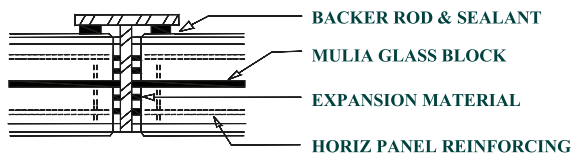
Jamb - Detail of Steel Dividers Between Horizontal Panels All Panels using Vertical Dividers should not exceed 10 ft. in height
